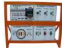
HB-P007S-TM TRAINER PLC SIEMENS S7-1200
